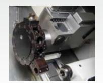
Radial Driven Tool BMT tooling system
