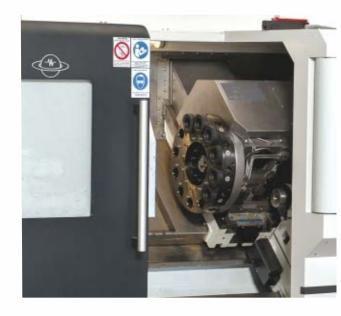
All structural parts are manufactured from high quality Meehanite cast iron and stress relieved for deformation.
